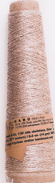
Silk wrapped around stainless steel 69% silk, 31% stainless steel
