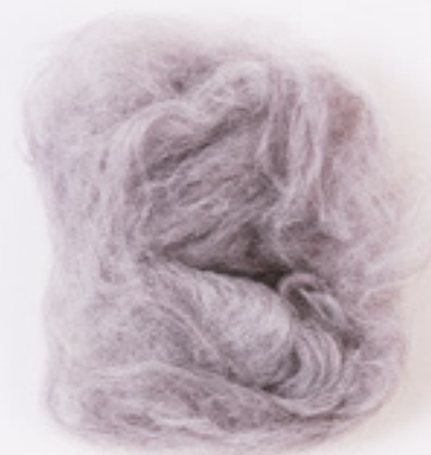
Stainless steel fibers blended with polyamide fibers
