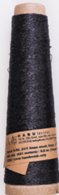
Linen wrapped around stainless steel 83% linen, 17% stainless steel
