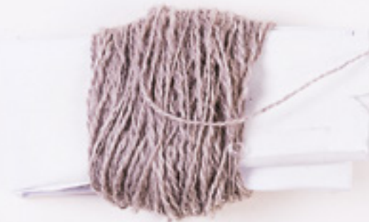
Hand-spun yarn from stainless steel- polyamide blend
