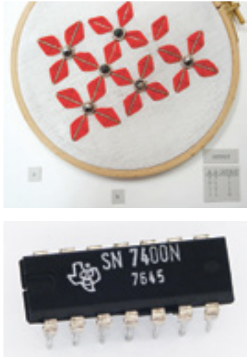
Figure 2 Above: XOR Gate, hematite beads, metal thread, silver paint, and cotton, embroidered. Photograph by Irene Posch. Below: 7400 chip, PDIP packaging, manufactured by Texas Instruments. The chip is approximately the size of a single bead used in the embroidery pictured above. Image from Wikimedia Commons, Stefan506.
